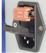
Fig. 5: Fuse location on the rear panel and in the carrier (1 of 2 fuses visible)
